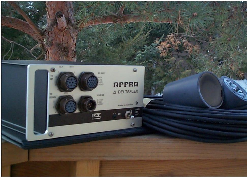
The Deltaflex is a fourth generation acoustic flowmeter and data recorder designed to measure direct velocity, reflected velocity, stage, discharge, temperature, salinity, speed of sound, receiver gain, and the ratio between the reflected and direct velocities.
